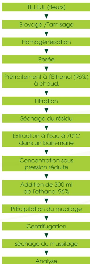
a hot plate stirrer. The extraction was carried out at 343.15 °K (70° Celsius) during 4 hours. After centrifugation (4,000 rpm for 20 minutes), in order to improve the yield from the mucilage extraction, the marc is washed with 50 ml of distilled water. This enabled us to increase the yield. The washing solution is added to the extraction solution. The extracts were combined, concentrated was done below 333.15 °K (60 °C) with a rotary flash evaporator under reduced pressure.
